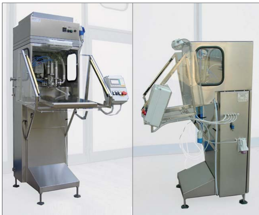
Fig. 1: Semi-automatic filling stations – here the model Liquiwell Filler BiB Italy – pump fruit juice into the tubes. An inductive fluid measurement ensures – depending on the volume of the bag – an optimal filling. (© Liquiwell)
